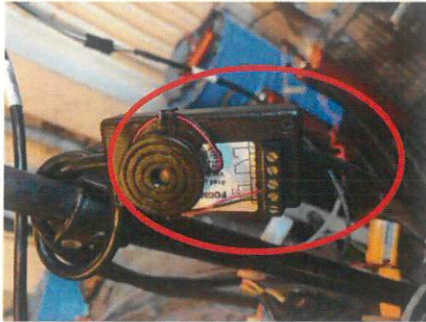
Control Panel (Buzzer, Activation Switch and Visual Signal)
